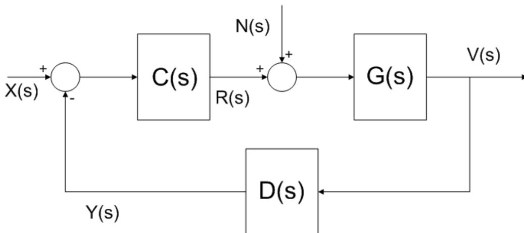
Figure 5: A model for the cruise control system.
