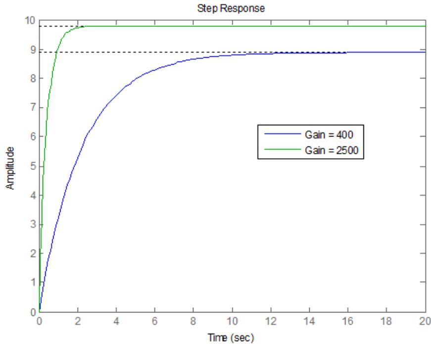
Figure 4: A plot of  $v(t)$ . This is the closed loop response of the system for gains ( $K_p$ ) of 400 and 2500.
