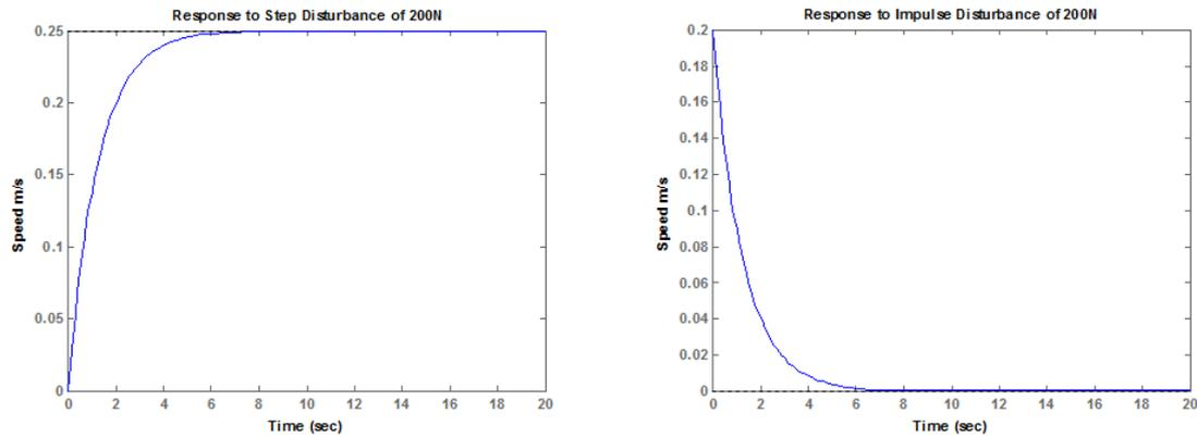
Figure 6: The step (left) and impulse (right) response to a wind force of 200 N. *i.e.* The input signal on the left is  $200u(t)$  and on the right is  $200\delta(t)$ .
