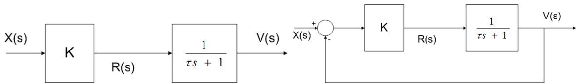
Figure 9: Block Diagrams for open and closed loop 1st Order systems with a proportional controller.
