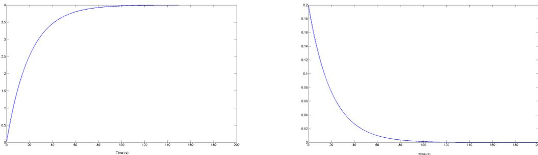
Figure 8: The step (left) and impulse (right) response of the open loop system to a wind force of 200 N. *i.e.* The input signal on the left is  $200u(t)$  and on the right is  $200\delta(t)$ .
