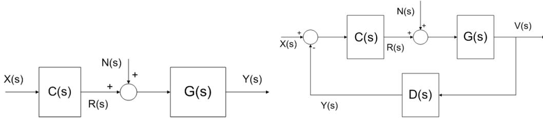
Figure 11: Open and Closed loop Models for disturbance inputs.
