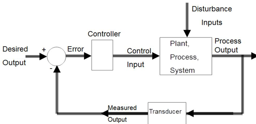
Figure 1: A basic Control System Architecture
