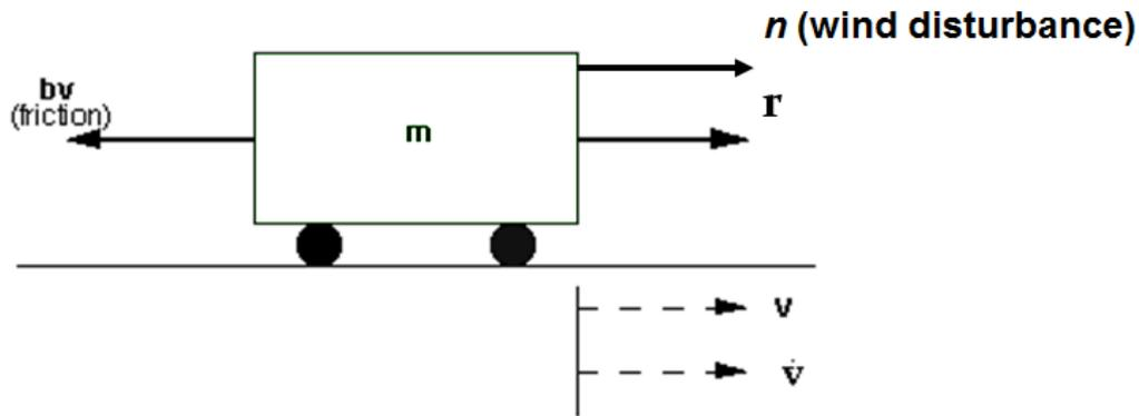
We will now see how our system responds to a buffet of wind. The wind is modelled as adding an extra force  $n(t)$  to the car. Hence we can modify our control system model as follows
