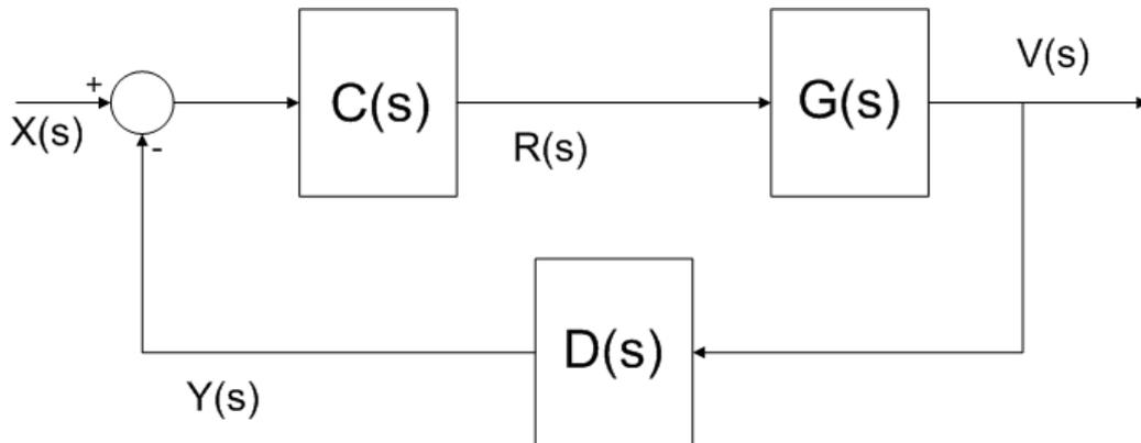
Figure 3: A model for the cruise control system.
