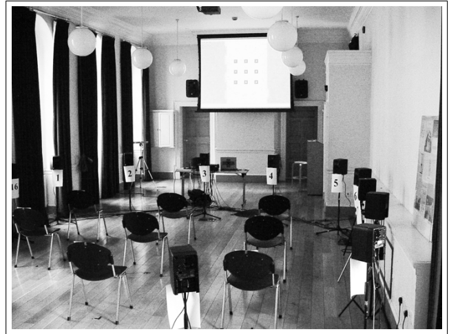
FIG. 1. Printing House Hall in Trinity College Dublin showing listener/loudspeaker setup.
