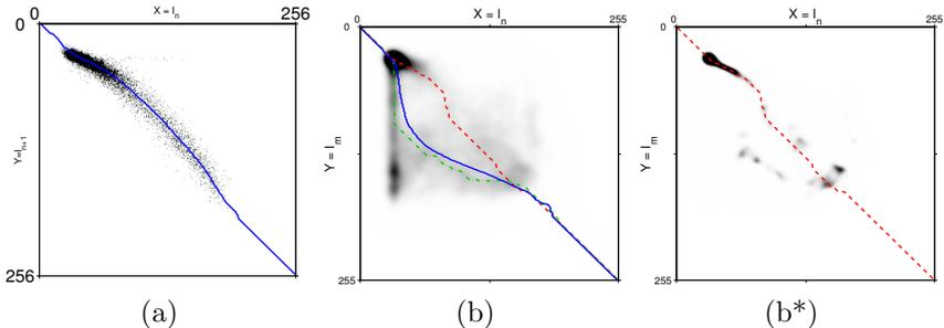
**Fig. 3.** Examples of joint pdf and their corresponding estimated distortion functions. On (a) an example of non linear distortion and its pdf matching estimation; on (b) an example of blotch noticeable by the vertical line and its consequence on the estimation by pdf matching (solid blue), by using MAP (dotted green) and by using the inlier enhancer and MAP (dashed red); on (b\*): the joint pdf of (b) after inlier enhancement.
