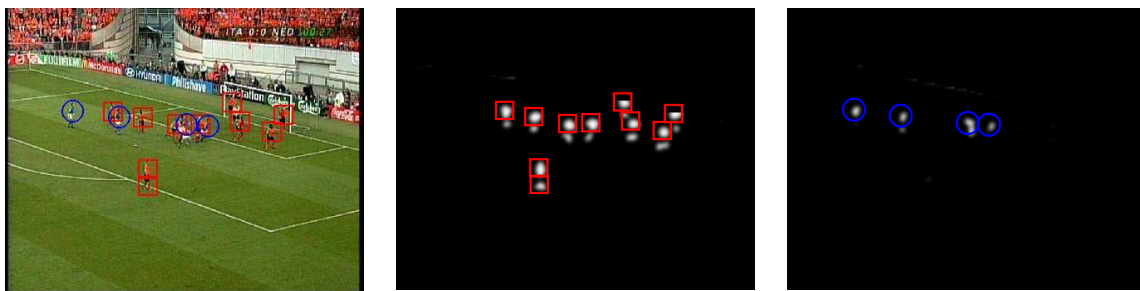
Fig. 3. Example of Player Detection using colour segmentation and MeanShift to find the blobs centres.
